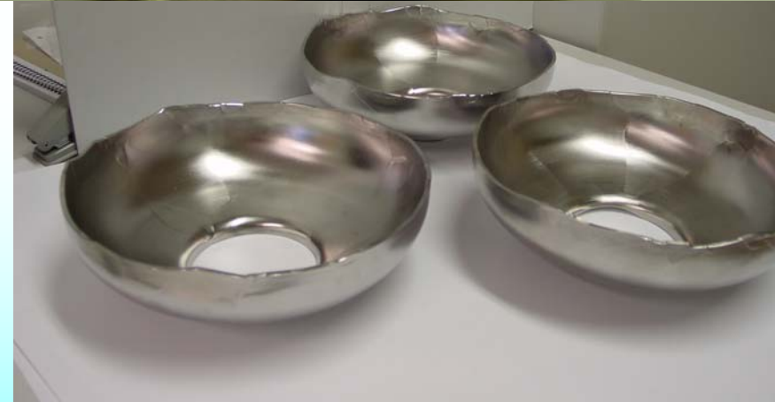
Deep drawn half cells of Ningxia LG Nb; necking of the wall thickness at iris on grain boundaries
